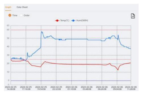
Click the "Graph" tab to display currently selected data of the logger. It can be the data of a currently connected logger or the historical data stored in the database.
